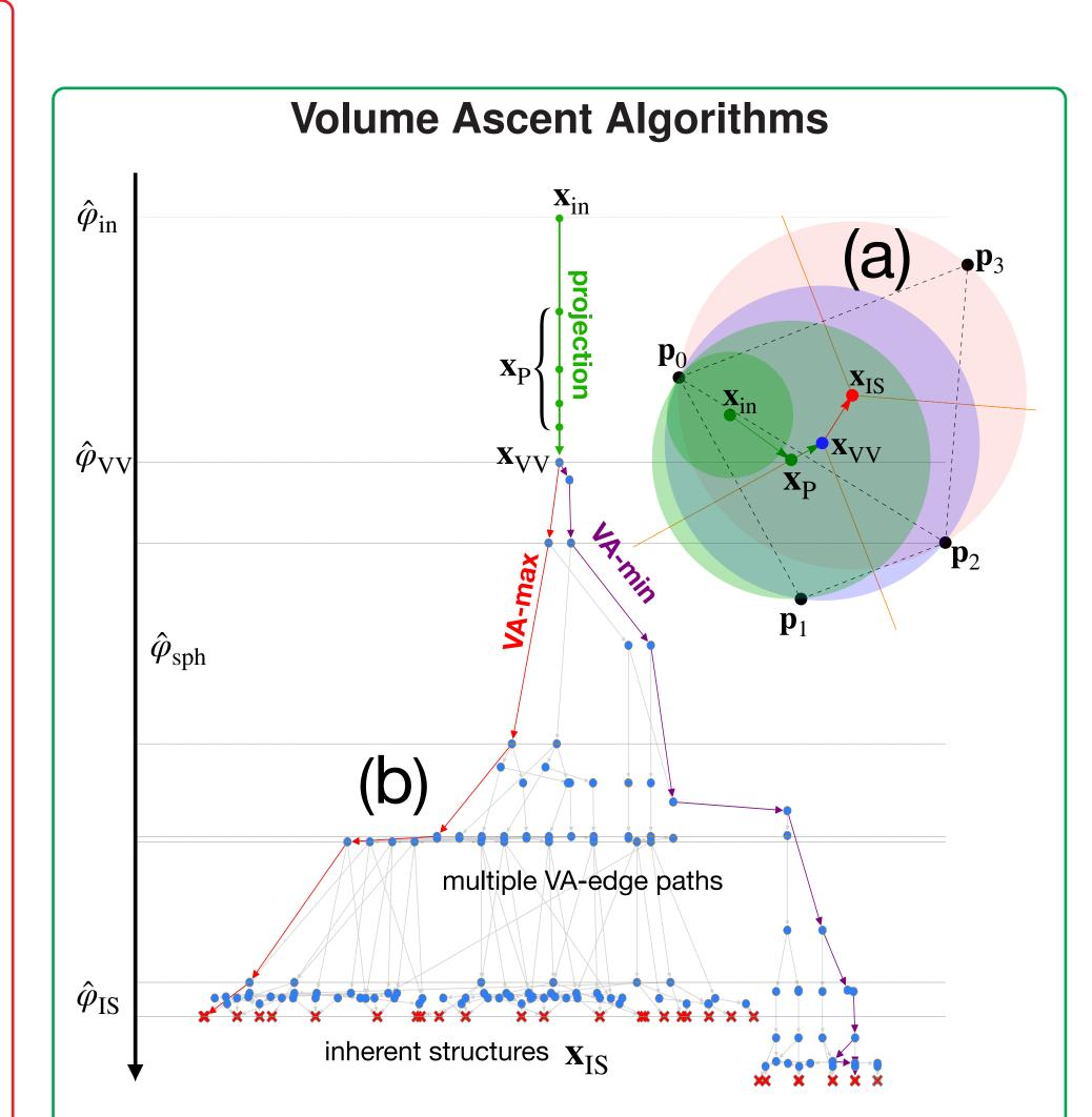
Despite the rarity of stable DS, VA algorithms can still reach them efficiently by monotonically increasing the tracer radius  $r_{\rm sph}$  (a). These schemes evolve a non-smooth, kinked landscape, for which standard optimization fails. Each unstable **Delaunay simplex** is associated with a Voronoi vertex (VV) and a cone of ascent directions.
