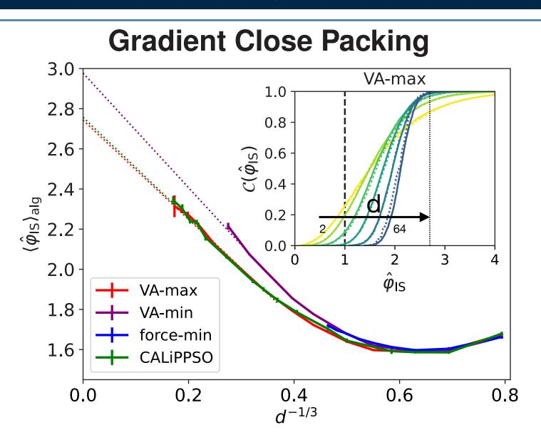
VA-max and CALiPPSO [5] reach similar jamming densities, scaling as  $d^{-1/3}$  and converging to  $\hat{\varphi}_{\mathrm{J}0} \approx 2.73$  as  $d \to \infty$ . In contrast, VA-min and force-min achieve denser packings ( $\approx 2.94$ ). The distribution of  $\hat{\varphi}_{\rm IS}$  sharpens with increasing d.
