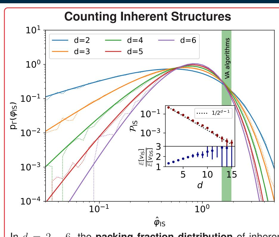
In d=2-6, the packing fraction distribution of inherent structures (ISs) follows a Gamma law (full lines), peaking at (d-1)/d with power-law left and exponential right tails (dotted lines are numerical results). The *mean packing fraction* is 1 in all d, but **VA algorithms** typically reach higher values. Each IS is the circumcenter of a stable Delaunay simplex. In high d, stable DSs (aka ISs) are **exponentially rare** — both in number and in volume.
